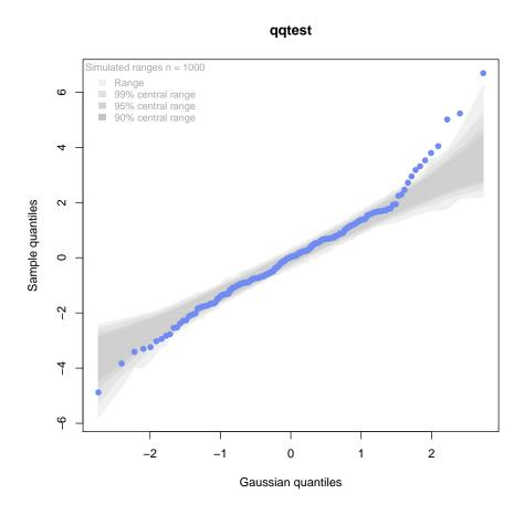
Here the points should follow a straight line and be within the shaded area. We could reject (A4) but accept (A4-bis) in the case where deviation to the straight line mostly arise in the tails. Statistical test (like a shapiro test) are not recommended since they do not enable us to know whether we reject (A4) or (A4bis).
