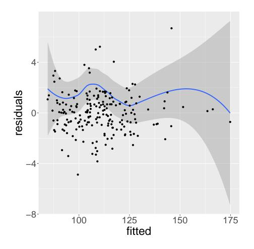
(see also the function **spreadLevelPlot** from the car package). It is also possible to have a global statistical test (Breusch-Pagan test):
